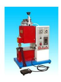
This Machine is used for coating glue onto plane material with different thickness in shoes-making, packing industry, wooden-processing, toy, leather, zipper-making, Clothing and electronic, etc, it can substitute double tape(to avoid unnecessary separating-paper)and has features as cost saving and environment friendly.
